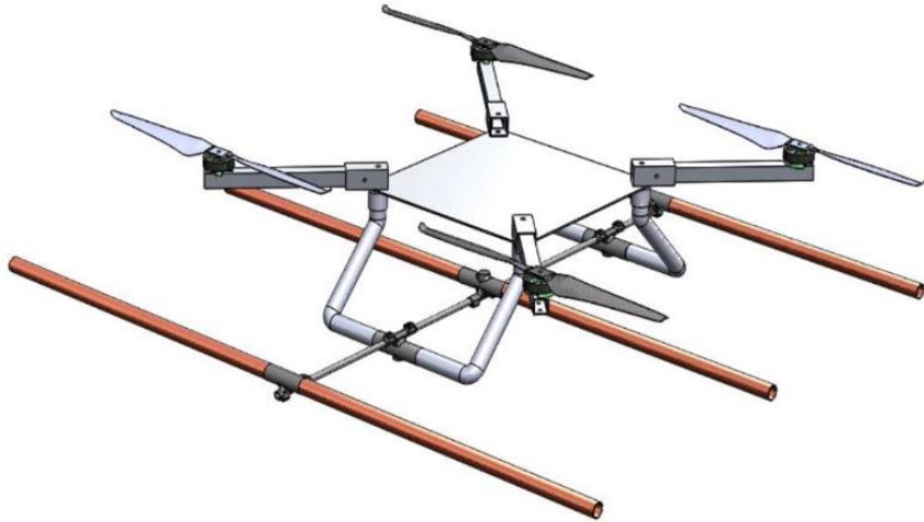
Figure 4: SolidWorks Assembly of Iteration 1.
